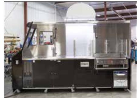
storage and mobility, and will also ensure that any venue employee, regardless of their stature or physical strength, will be able to comfortably lift and lower the canopy or header without assistance. Furthermore, if the carts need to be transported from one venue to another, the header or canopy will not have to be fully removed and reattached, thus saving the venue time and money on costly labor.
